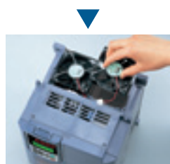
Disconnect the power connector and change the cooling fan cartridge.
