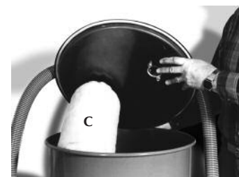
(A) Vacuum flow from receiver to blower; (B) Vacuum flow to receiver; (C) Filter
