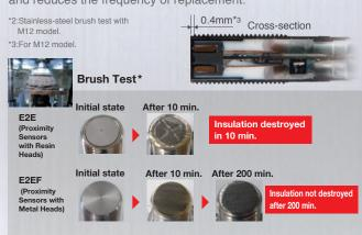
\*Test results for stainless-steel brush rotating at 130 rpm.
