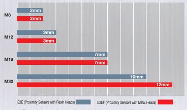
\*1:The actual sensing distance will vary with the size or material of the object. For details, refer to Engineering Data.
